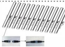
7.Connect the waterproof connector on the light bar to the main beam assembly connector and lock the waterproof connector.
